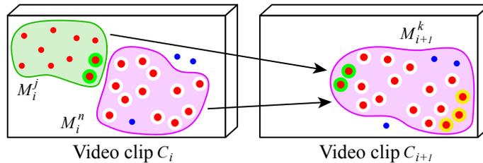
Fig. 4: Trajectory counting between two connected motions. Green circles: shared trajectories between  $M_i^j$  and  $M_{i+1}^k$ . White circles: shared trajectories between  $M_i^n$  and  $M_{i+1}^k$ . Yellow circles: newly appeared trajectories in  $C_{i+1}$  that belong to  $M_{i+1}^k$ .
