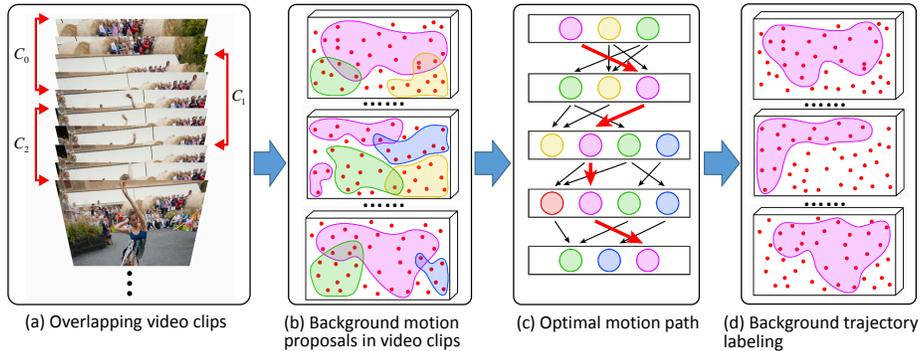
Fig. 1: Pipeline of our background feature identification method. (a) Divide sequence into multiple overlapping clips  $\{C_i\}$  Red points in (b) and (d) are feature trajectories in video clips. Red arrows in (c) is the global dominant rigid motion that contains the largest amount of feature trajectories.
